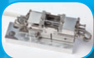
"Anti-stick" carbon evaporator source, designed to accept 6.15mm diameter carbon rods. Four springs maintain an even pressure during the evaporation process and ensure even, reproducible deposition
