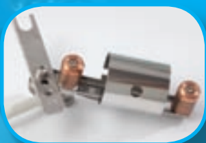
The standard metal source can be used to evaporate a range of metals from a suitable tungsten filament or boat. The terminals can also be used to evaporate carbon fibre. An adjustable source shield is fitted to help maintain the cleanliness of the system
