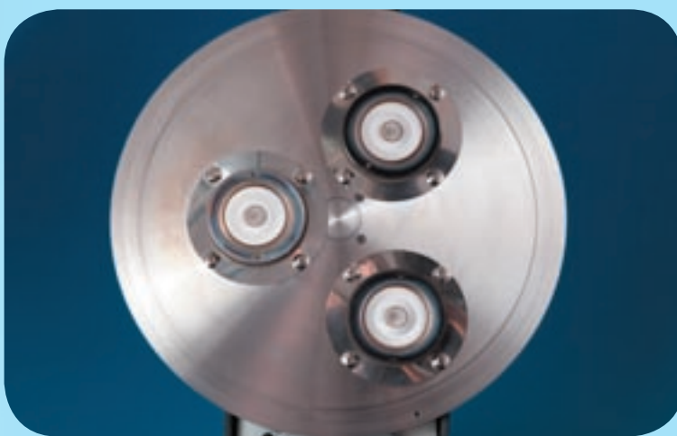
Triple sputter head with automatic shutter control
