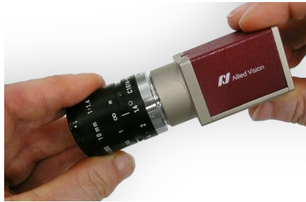
Figure 43: Illustration of camera orientation when removing lens or dust cap
