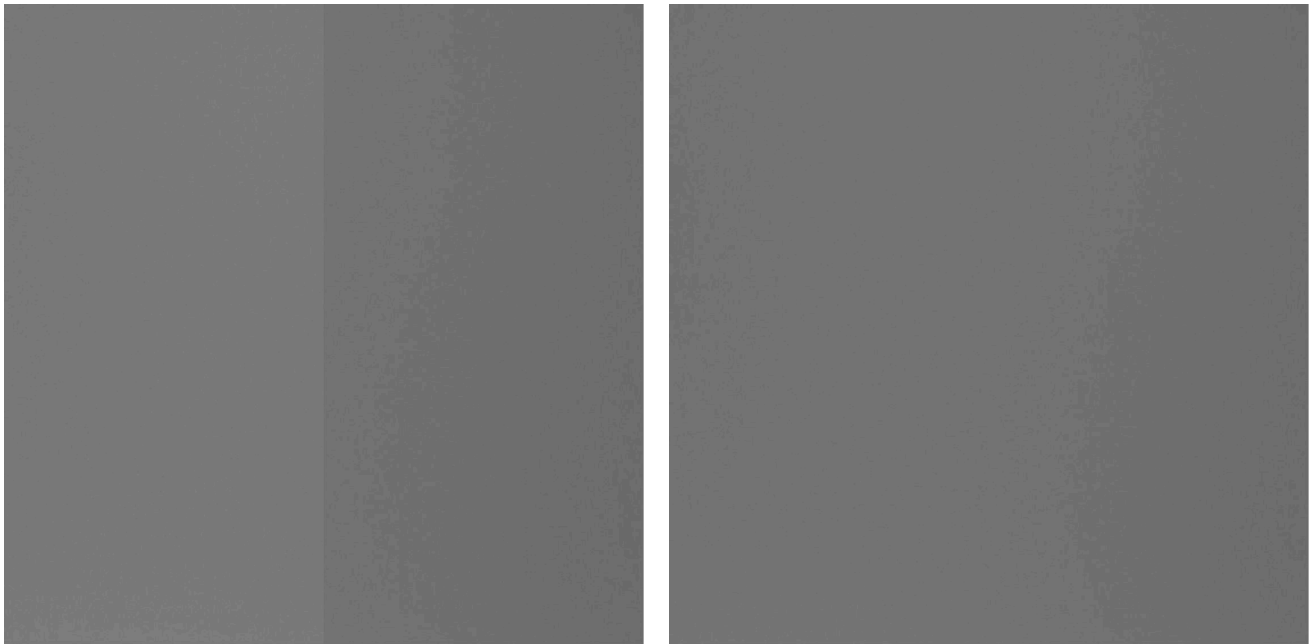
Figure 89: 2-Tap Sensor - Unbalanced image (left) and matched image (right)
