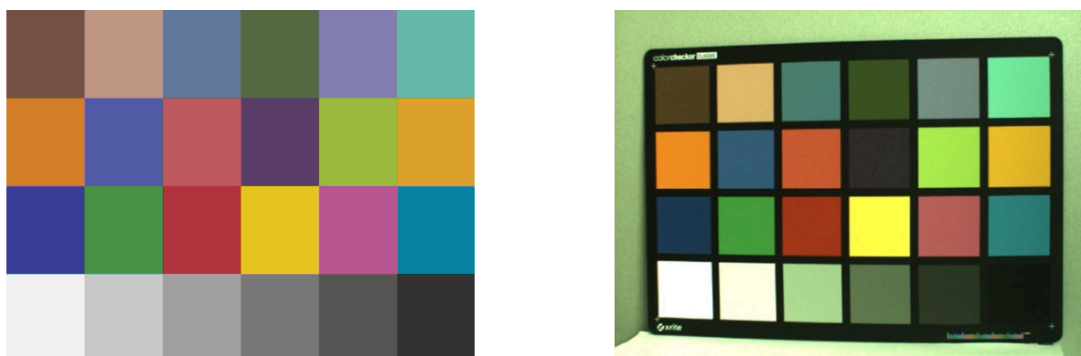
Figure 150: Comparison original color (left) and camera image (right) of a ColorChecker chart
