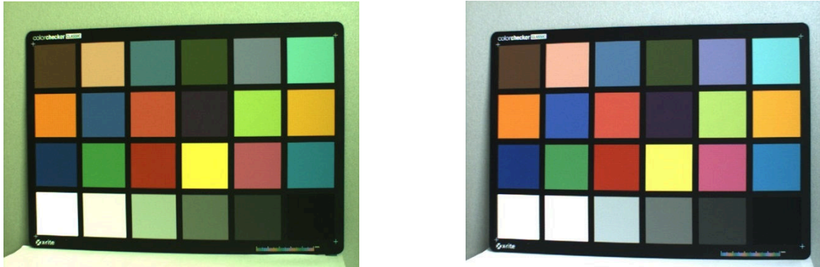
Figure 151: ColorChecker chart without (left) and with White Balancing (right)
