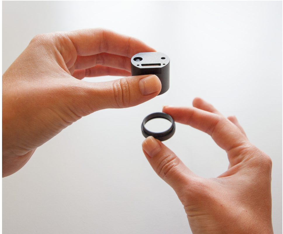
FIGURE 8.4 Camera Positions before Screw in and Screw out of the C-mount Adapter, Lens, or the Camera's Cover
