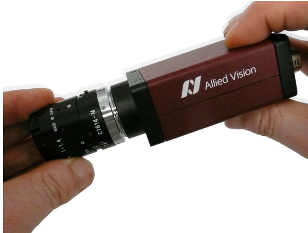
Figure 101: Illustration of camera orientation when removing lens or dust cap
