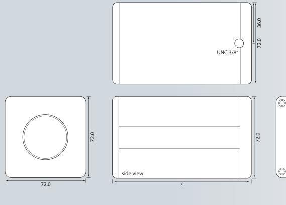
x = Lenght (standard): 122 mm Length (with CF interface): 137 mm Length (with Video Interface): 129 mm Length (with CF- and Video Interface): 144 mm
