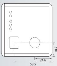
$\label{eq:longth} \begin{subarray}{ll} Length (standard): $x = 122 mm, $y = 118.5 mm$\\ Length (with CF interface): $x = 137 mm, $y = 133.5 mm$\\ Length (with Video Interface): $x = 129 mm, $y = 125.5 mm$\\ Length (with CF- and Video Interface): $x = 144 mm, $y = 140.5 mm$\\ \end{subarray}$
