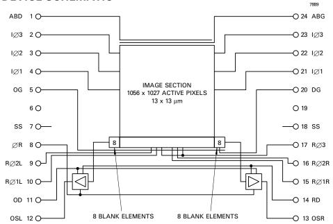
**Note** Pins 6 and 19 are not connected. For convenience, the CCD47-10 Compact Pack is pin compatible with the e2v technologies CCD57 sensors in the compact pack, except that OSL = pin 6, OSR = pin 19 and pins 12 and 13 are not connected in the CCD57.
