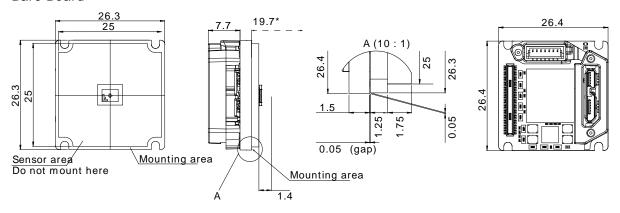
$<sup>^{\</sup>star}$ Mechanical length for C-Mount, for other mounts and details, see the user guide.
