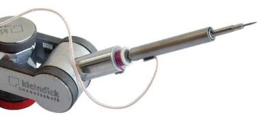
Standard tungsten probe tips can be inserted into the front of the axis and rotated with a resolution of o.1° per step, allowing applications like true FIB lathe milling, tomography and STEM to be performed with ease. In addition the MGS2-EM microgripper can be combined with the rotational tip to allow gripped objects to be rotated.
