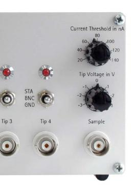
The STA offers a valuable time reduction and greatly reduces the risk of damaging the probe tip and the sample when approaching a region of interest. It can also be used to test the resistance of contacts e.g. the drain of an FET.
