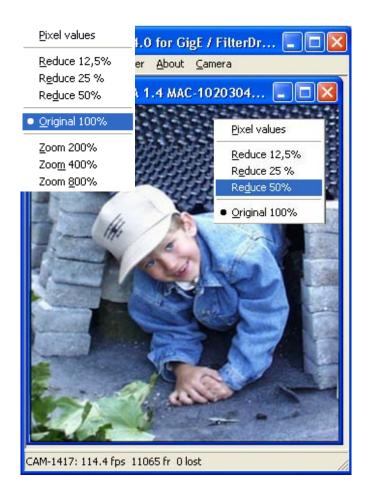
If "Pixel values" is selected the display switches in the bottom left corner to displaying the min and max values at cursor position along with the difference max-min which represents the image's noise amplitude at cursor position:
