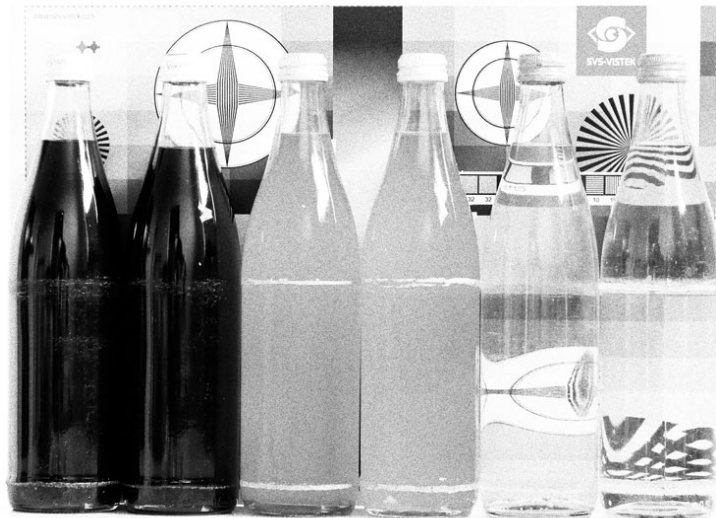
Figure 27: noise caused by increasing gain excessively
