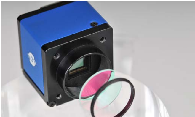
Figure 74: Figure of ECO standard & ECO Blackline - without and with IR cut filter
