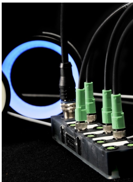
Figure 57: use the breakout box to simplify your wiring
