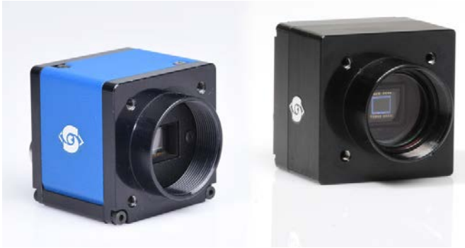
Figure 76: ECO standard & ECO Blackline with IR cut filter
