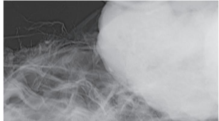
Plastic foam: 60kV, 2micron resolution
