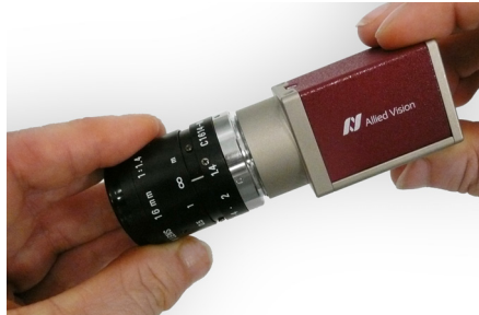
Figure 44: Illustration of camera orientation when removing lens or dust cap
