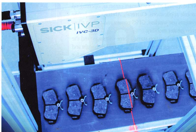
ABOVE: The IVC-3D from Sick, inspecting brake pads. FAR LEFT: Possible underdrawings on the Mona Lisa, studied by XenICs systems. LEFT: A ceiling tile, inspected using Fraunhofer's systems.
