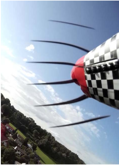
Figure 14: Rolling shutter with fast moving object details
