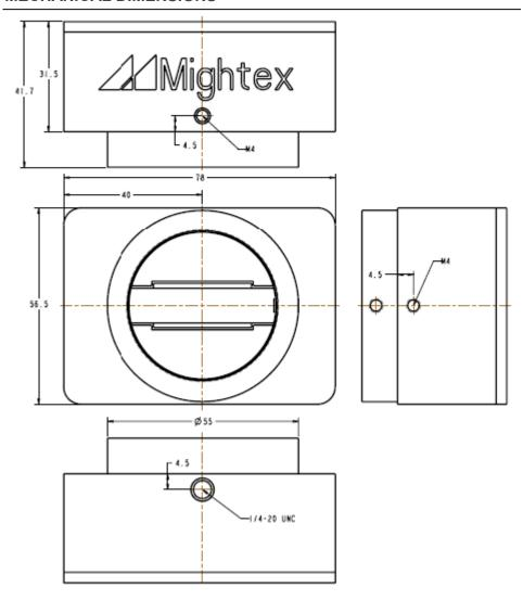
Length x Width x Height: 78(mm) x 42(mm) x 57(mm) Weight: 200g
