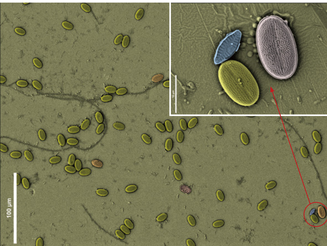
日立 FlexSEM, 5kV, WD 5.9 mm, x200, SE
