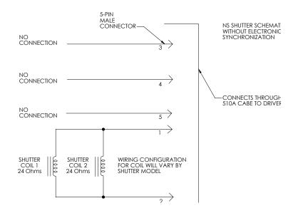
The schematic to the left illustrates the wiring for the NS65B. The schematic also shows the two 24  $\Omega$  coils wired in parallel to provide an equivalent resistance of 12  $\Omega$ .
