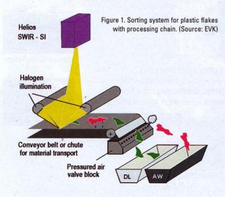
extremely small image capture units. As a consequence, system designers have a lot more freedom in finding the optimal layout for efficient separation and sorting systems.
