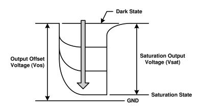
xiii Difference between output reference voltage and absolute output voltage with an integration time of 25 ms.
